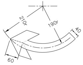
The centre line of the arrow head is angled from the outside arc of the shaft to the centre line arc of the shaft.
