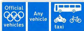
ORN 3.2.13 (959) – Nearside games lane, central lane for any vehicle and offside bus, m/c, cycle and taxi lane repeater
