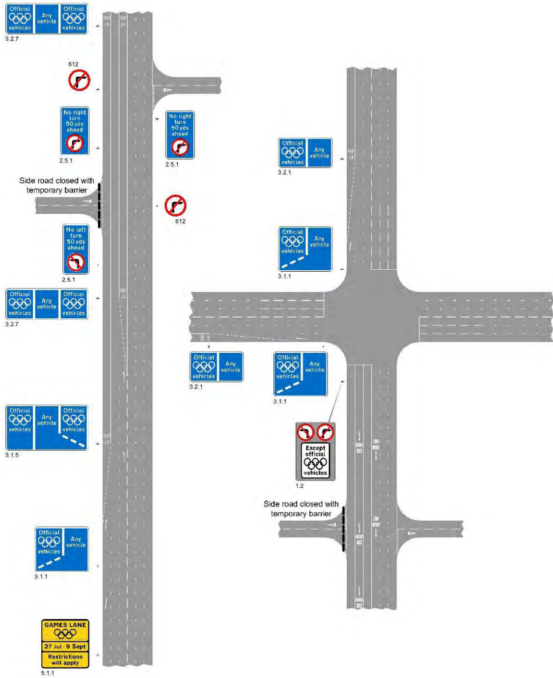
Figure 13 6 lane single carriageway Lane 1 - Games lane (turning left) Lane 2 - Any vehicle Lane 3 - Games lane (continuing ahead)
