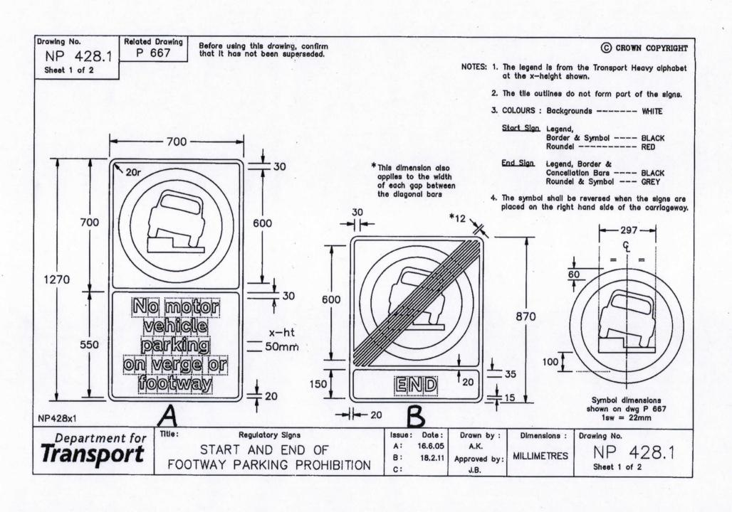
Drawing No. Related Drawing Before using this drawing, confirm that it has not been superseded. (C) CROWN COPYRIGHT P 667 NP 428.1 NOTES: 1. The legend is from the Transport Heavy alphabet. Sheet 2 of 2 The tile outlines do not form part of the signs. COLOURS : Backgrounds ---- WHITE Start Sign Legend,
