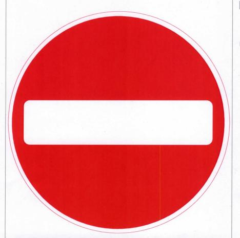
Scale 1:6 Dimensions (in mm): Width: 750, Height: 750 Width: 745, Height: 390 x-Height: 50 Area: 0.73 sq m
