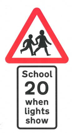
This would be used above light signals to diagram 4004 Dimensions assume speed limit of 30mph Sign diagram 545 – 600mm Plate 50mm x-height except "20" at 100mm x-height .
