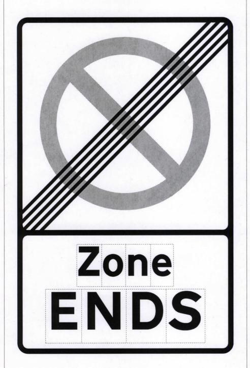
Scale 1:5 Dimensions (in mm): Width: 570, Height: 875 x-Heights: (37.5), 55, 70 Area: 0.50 sq m
