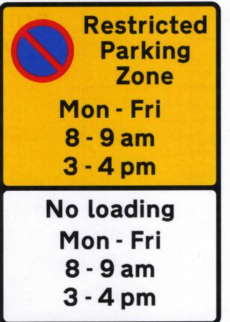
Dimensions (in mm): Width: 441, Height: 639 x-Height: 25 Area: 0.28 sq m Colours: black on yellow black on white Drawing Title: Drawn by: Checked by: Quantity required: \_ [ ] Single Sided [ ] Double Sided Class 1 retroreflective with: [] Channels [ ] Offset brackets [ ] Bracketed chevron end All signs to be manufactured in accordance with BS873 Slough Borough Council **Transport Development** P.O. Box 580 Wellington House **High Street** Slough SL1 1FB www.slough.gov.uk
