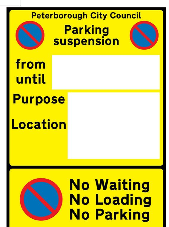
Sign to be illuminated by means of retroflective material to BS EN 12899-1 (2007) Class RA1
