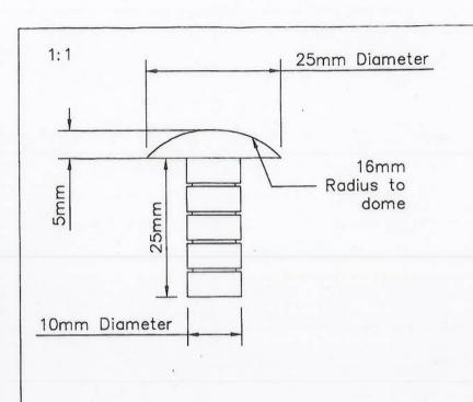
Domes are spherical with a flattened top. Stud to be fabricated in Stainless Steel. **Department for Transport**
