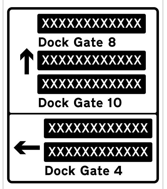
Scale 1:18 Dimensions (mm): Width: 2325, Height: 2690 x-Height: 100 Area: 6.25 sq m
