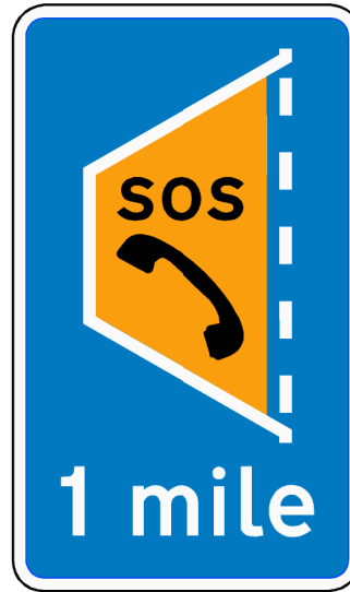
Sign Ref : ERA A1 Not illuminated The distance must be expressed in miles denoted by "mile(s)" and must be "1 mile" (unless site specific constraints necessitate variation.)
