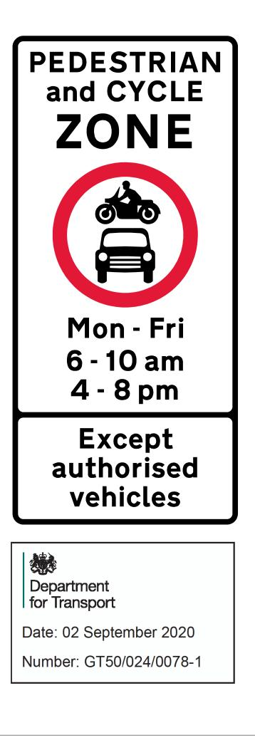
Scale 1:7 Dimensions (mm): Width: 582, Height: 1263 x-Heights: 37.5, 62.5 Area: 0.73 m<sup>2</sup>
