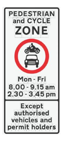
FACING Background: white/white Border size (mm): 14.06 Border colour: **BLACK** TEXT Style: Transport Heavy Colour: **BLACK** Lowercase(xheight (mm)): 37.5 Capital height (mm): 52.5 DIMENSION Width (mm): 600 Height (mm): 1355 Area (sq.m): 0.813 Tolerance:+ 5mm
