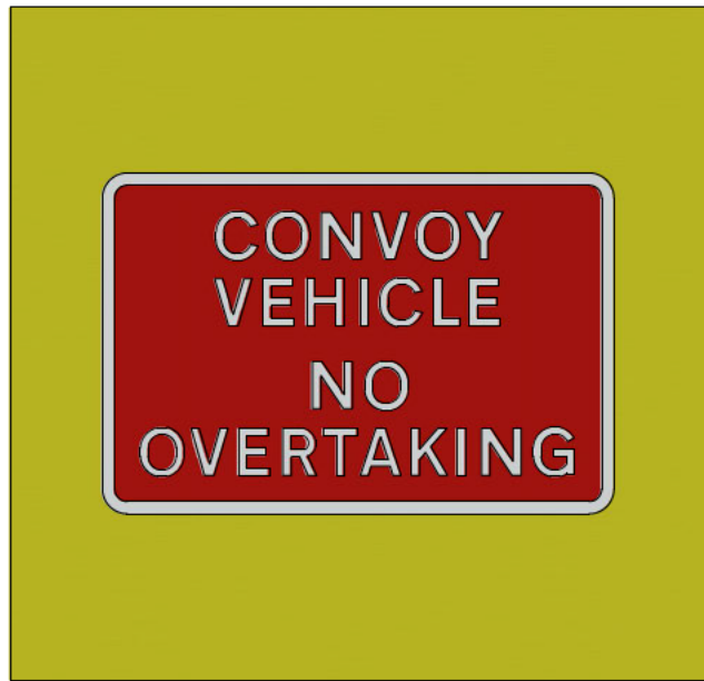
Aspect A Sign for Mobile Carriageway Closure
