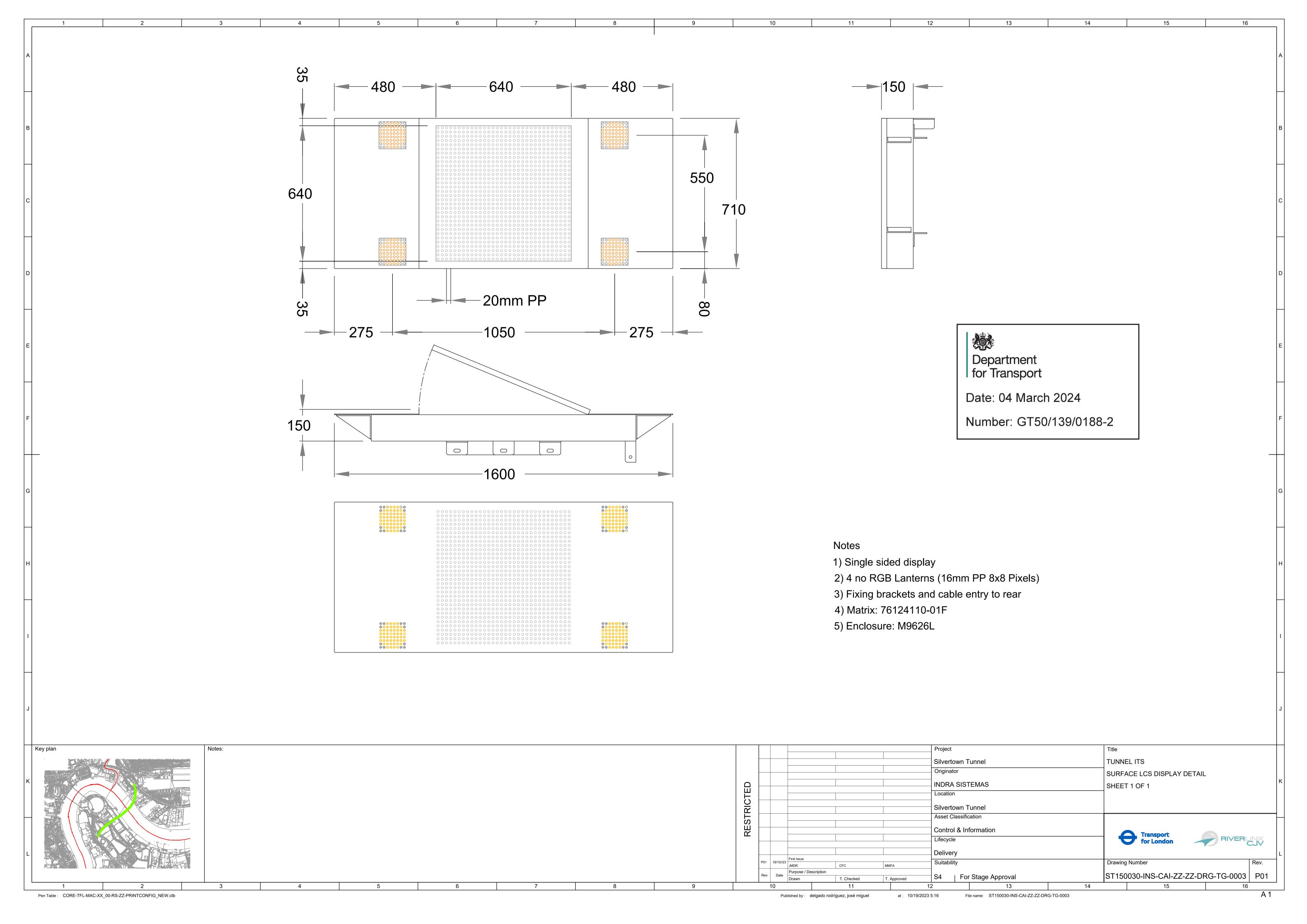
1610mm maximum Lantern centres 1050mm (nominal) Aspect Display Area 640mm (nominal) 550m Aspect Display Area 640mm (nominal) 715m 4 No. 125mm diameter Dual Colour - Red and Amber (Yellow) Lanterns Corner radius optional from 0 to Matt Black "Target Board" Surround 150mm
