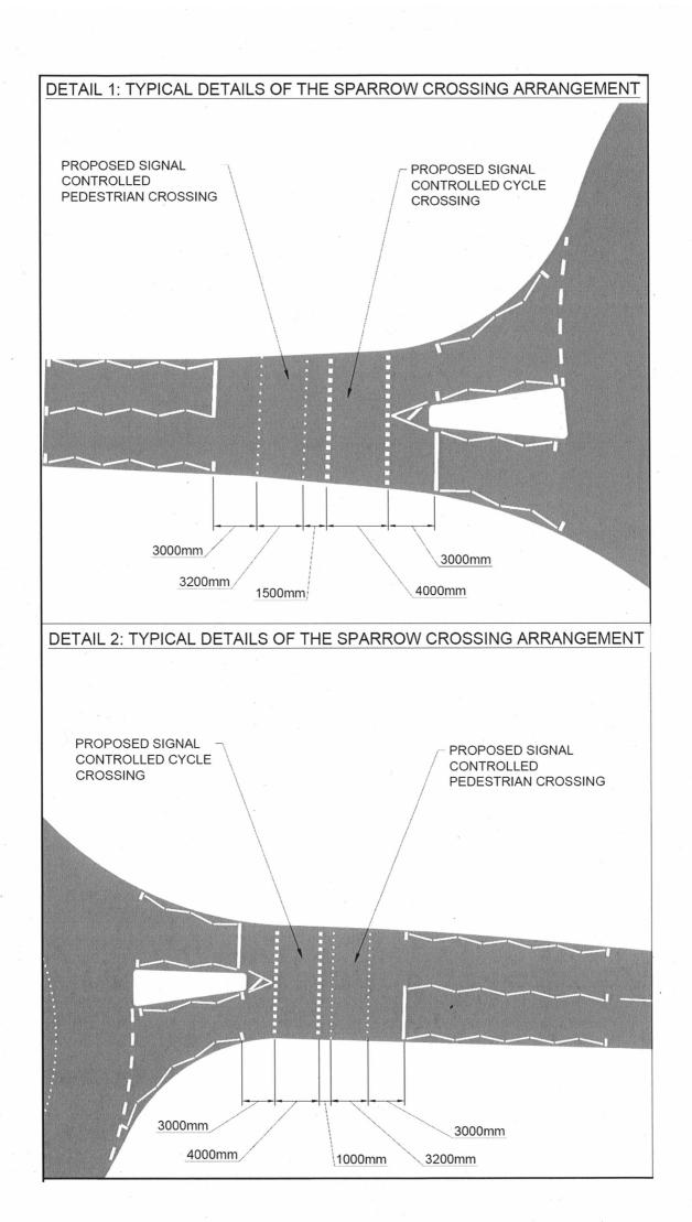
DETAIL 1: TYPICAL DETAILS OF THE SPARROW CROSSING ARRANGEMENT
