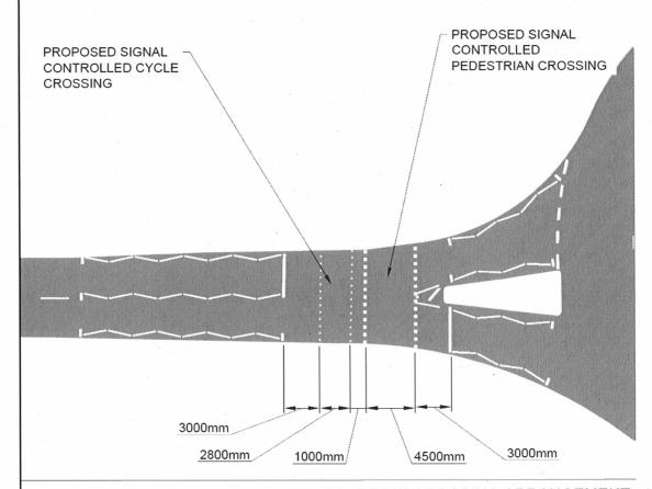
DETAIL 2: TYPICAL DETAILS OF THE SPARROW CROSSING ARRANGEMENT
