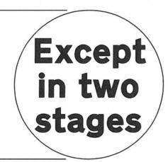
Text to be 35mm in height with font as specified in 'The Traffic Signs Regulations and General Directions 2002
